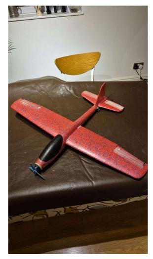
Wing dihedral removed and a carbon strip inserted along the length of the wing with hot glue Fuselage hollowed out using a knife and pliers, hinges for controls made from fibre parcel tape Wei 2600kv motor and a GN3 4s 1100mah battery, 40A ESC and a 5x4.5 3 blade prop Micro servos on each aileron and elevator is cut straight and rudder relieved for throw
