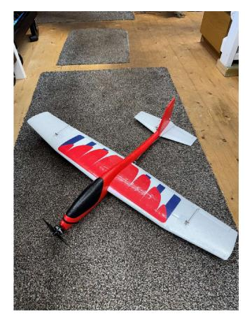
Wing dihedral left in place, stickers help to strengthen wing. Carbon tube set into rear fuselage for strength.
