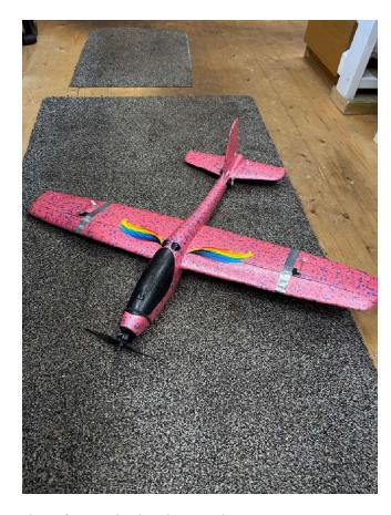
Wing dihedral removed and a carbon strip glued span of wing, carbon tube set into rear fuselage for strength.
