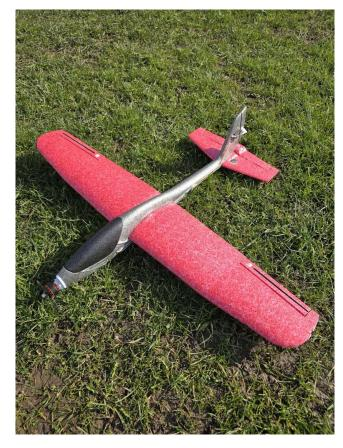
Wing with dihedral left in, carbon tube let into rear fuselage for strength.
