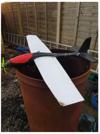
Wing with small amount of dihedral left in, carbon tube pushed into centre of rear fuselage for strength.
