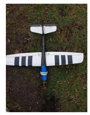
Original first release version. Wing with small amount of dihedral left in, carbon tube pushed into centre of rear fuselage for strength.
