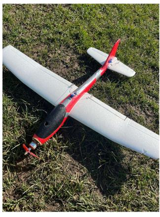
Wing with dihedral left in, carbon tube pushed into centre of rear fuselage for strength.
