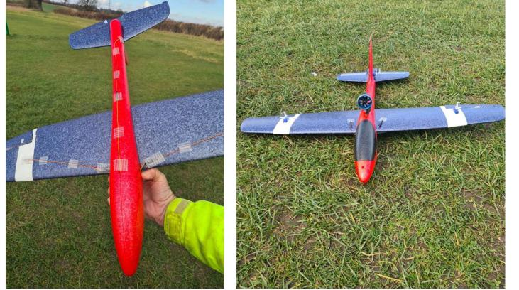
Wing dihedral removed by cutting and bending the wings.
