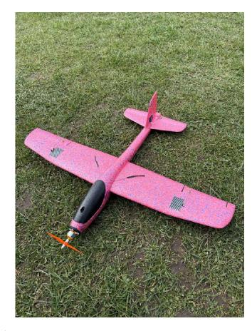
Wing dihedral left in place. Carbon tube set into rear fuselage for strength.
