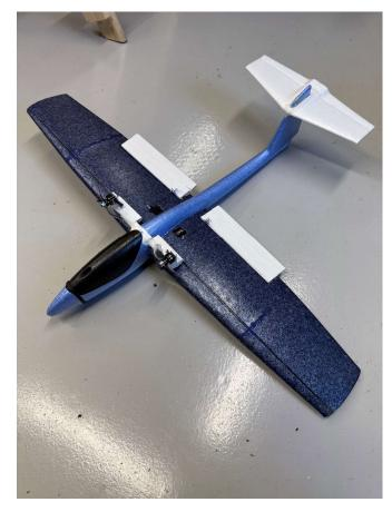
Wing dihedral removed and a carbon strip glued span of wing, carbon tube set into rear fuselage for strength and up into tail.
